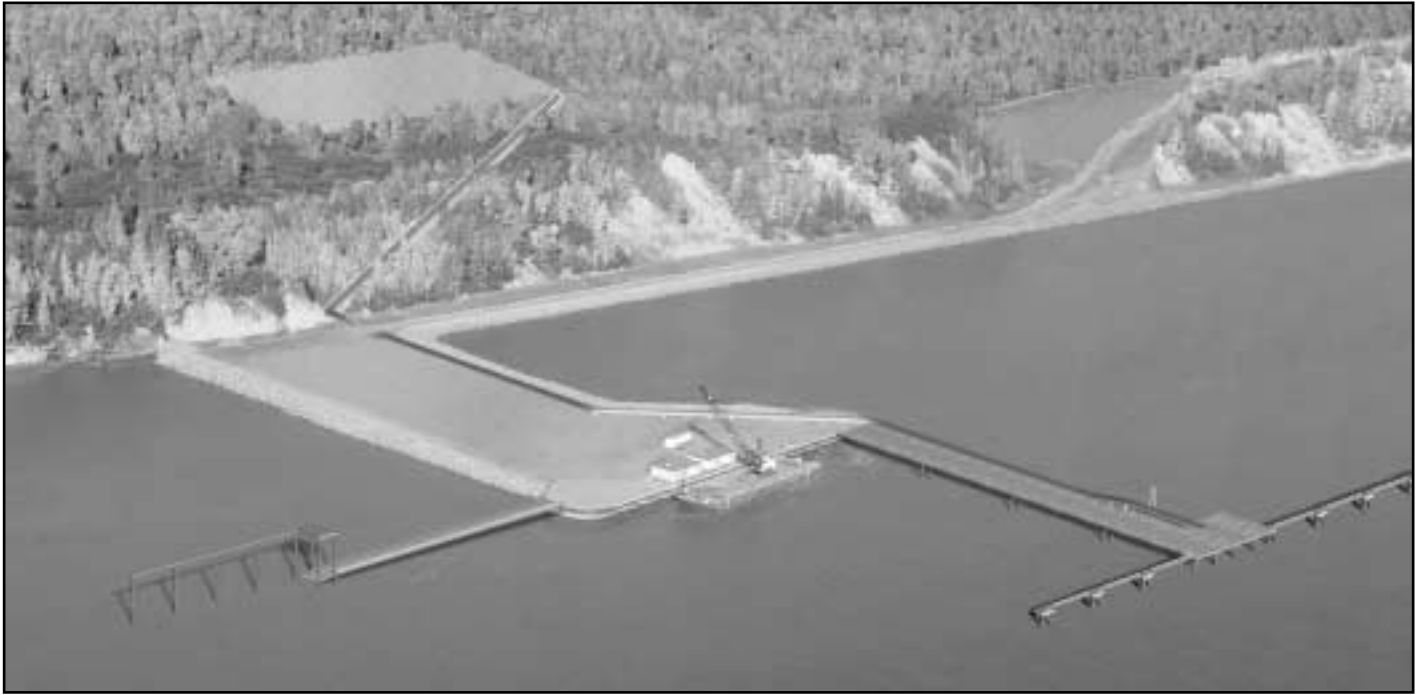
Digitally enhanced photo of Port MacKenzie illustrates the planned ferry vessel landings to the left of the existing barge dock. In the center, a crane is ready to load Alutiiq Manufacturing Company houses on a barge. Depicted on the right are the deep-water dock and the commodities conveyor, both planned for completion in 2004. Courtesy P N D Incorporated, Consulting Engineers.
